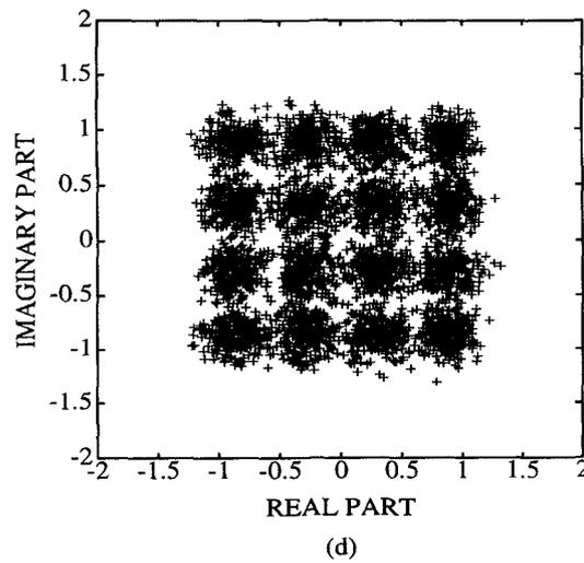
**Figure 1. (a) and (b) Unequalized signal constellations associated with  $x_1(n)$  and  $x_2(n)$ , respectively, for  $n = 0 \sim 4095$  and SNR = 20 dB; (c) and (d) equalized signal constellations associated with  $e_1(n)$  and  $e_2(n)$ , respectively, for  $n = 0 \sim 4095$  using the MS criteria with  $(s, l_1, l_2) = (1, 2, 2)$ .**
